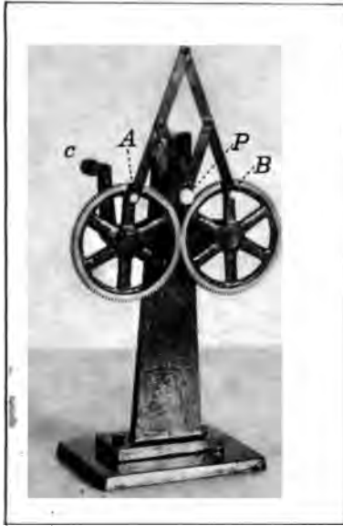
FIG. 8. Simple harmonic motion from mechanical movement.
